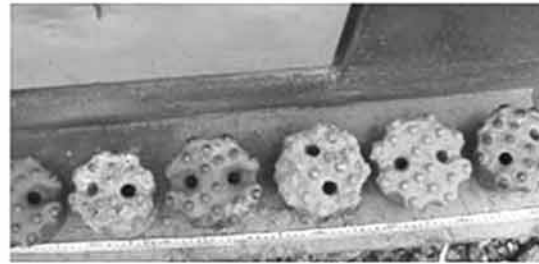
Figure 7: These bits were spotted in the bit-rack of a drilling rig in a gold mining operation. This is an example of the large range in bit sizes used by one driller on a single blast.
